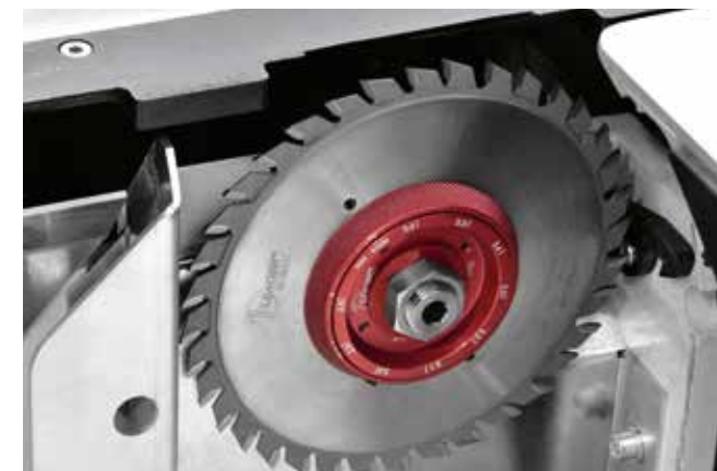
Expandable scoring blade Manually expandable with variable thickness from 2,8 to 3,6 mm. 120 mm blade diameter.
